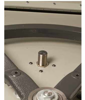
Safety Shutoff Sensor
