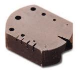
**SLOT ANVIL** These anvils have a flat smooth case hardened surface and can be used as a base for staking, riveting and drilling small parts. V-slot is handy for removing pinions and similar items. Has 9 graduated holes, with one size for stumps, and 5 milled slots. Measures 1¾" long, 1¼" wide and ½" thick.
